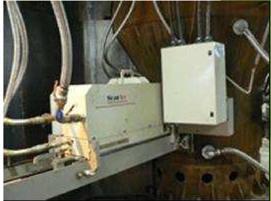
Gas Plasma Generator Attached to a Kiln
