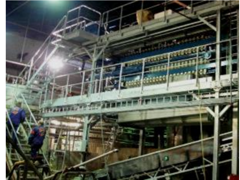
Production scale ~1-1.5 ton kraft lignin/hour
