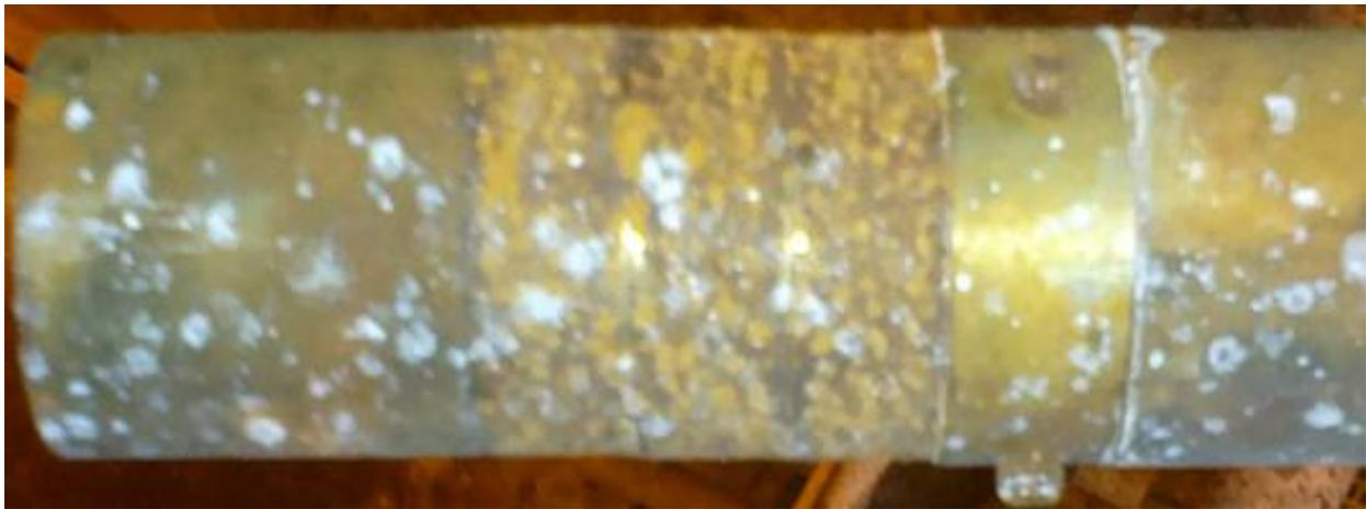
Figure 12. Probe after water wash - 1124h total (811h "normal" operation + water wash)
