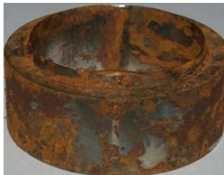
Figure 13. Ring after 1124h. Not that there are some areas without corrosion downwards on the bottom edge of the ring.
