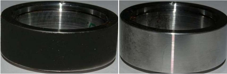
Figure 14. Ring after 2h exposure during oil burning.
