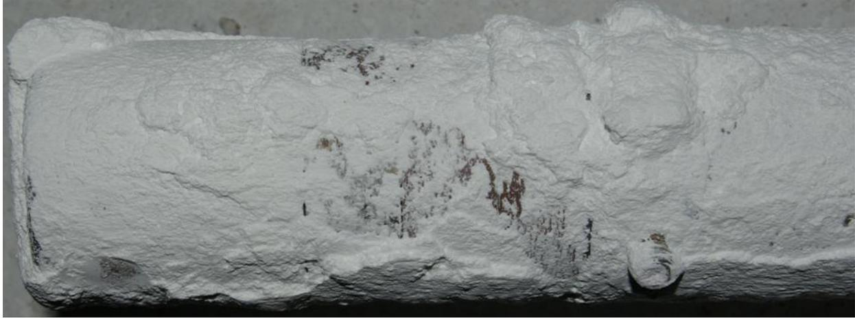
Figure 9. Probe after 811h of Normal Operation
