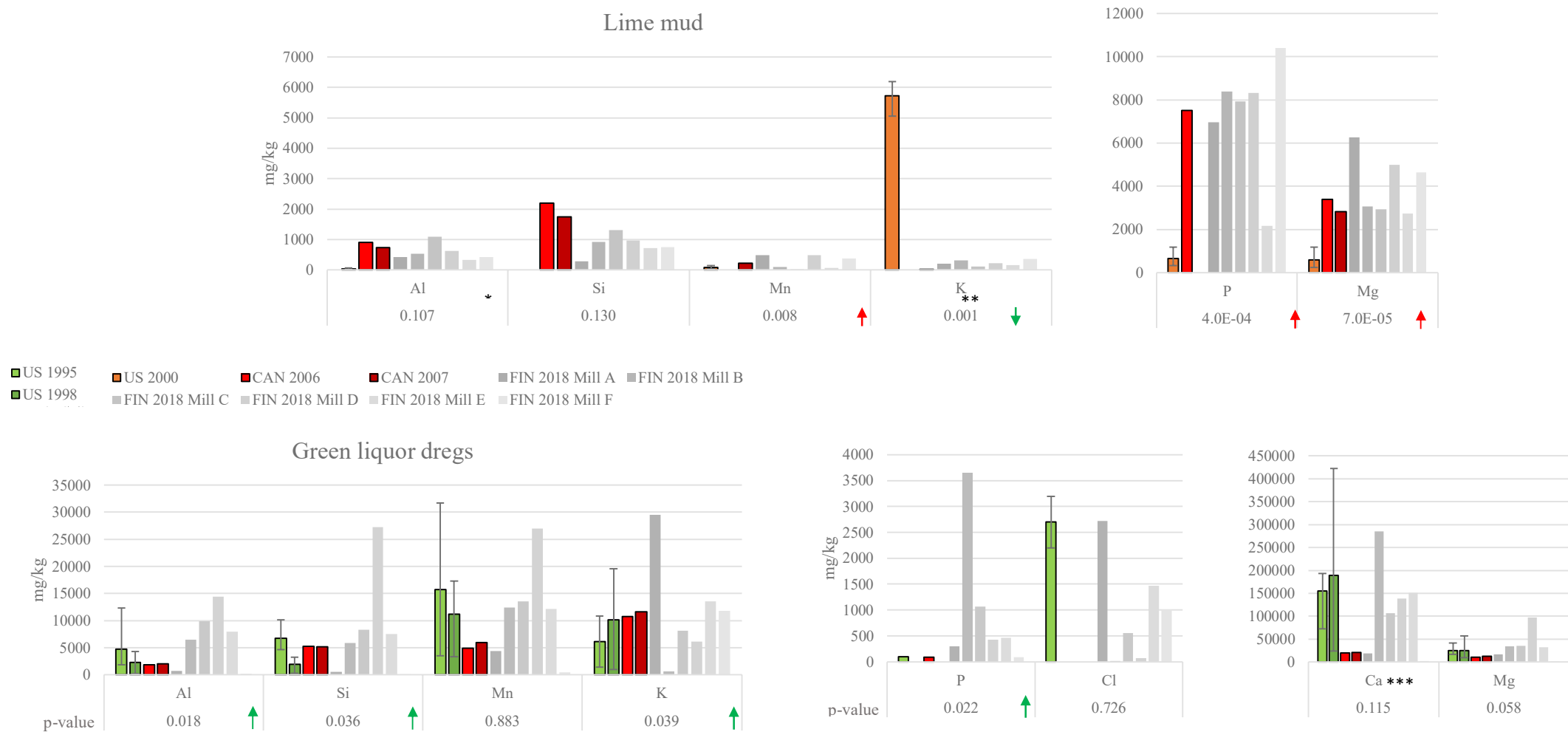
Figure 48 Lime mud and green liquor dregs comparisons between older North American results (Empie, et al., 1999) (Richardson, et al., 1998) (Frederick, et al., 2000) (Taylor & Bossons, 2006) (Taylor, 2007) and this project's results form 2018. The colored column represents the literature results. The error bars show the minimum and maximum values of the literature data. P-value of the t-test is shown in x-axis. Values under 0.05 are considered in this two-tail test significant. The green arrow indicates in lime mud that the newer values are significantly lower, and the red color indicates that the newer values are significantly higher. In green liquor dregs, the green arrow indicates that the newer value has higher NPE concentration. * The abnormally high Al values from Mill C are not included in the t-test. P-value was 0.037 with Mill C. ** The literature reference (Frederick, et al., 2000) has very high values in some of the sample points and has to be taken into account when analyzing the results. *** Mill B has lime mud in its green liquor dregs sample.
