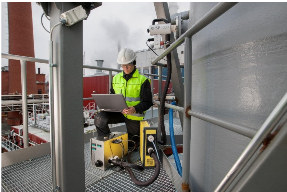
Figure 24 Above pictures A and B show how measurer works with the FTIR in some industrial flue gas (pictures from Gasmét Oy)
