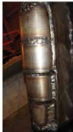
Probe before installation into liquor gun opening (MB Joutseno)
