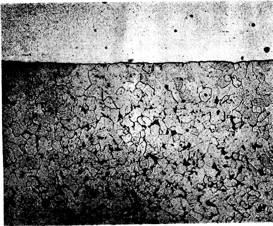
Figure 5 The bonding zone of the composite tube according to Figure 4. At the top the stainless steel, then the bond and a decarburized carbon steel zone. At the bottom the carbon steel. The condition similar to the installation condition. No disbonding has occurred.
