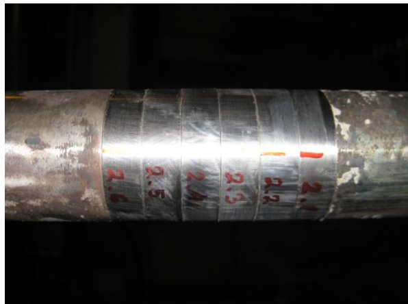
Figure 3. Attachment of the test material rings in the probes. Sample number 1.1(SAN 28) respectively 2.1(SAN 28) is farthest from, and Sample number 1.6 (347H) respectively 2.6 (347H) closest to the tip of the probe. Windward side is marked with red line.
