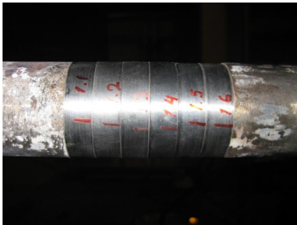
Figure 3. Attachment of the test material rings in the probes. Sample number 1.1(SAN 28) respectively 2.1(SAN 28) is farthest from, and Sample number 1.6 (347H) respectively 2.6 (347H) closest to the tip of the probe. Windward side is marked with red line.
