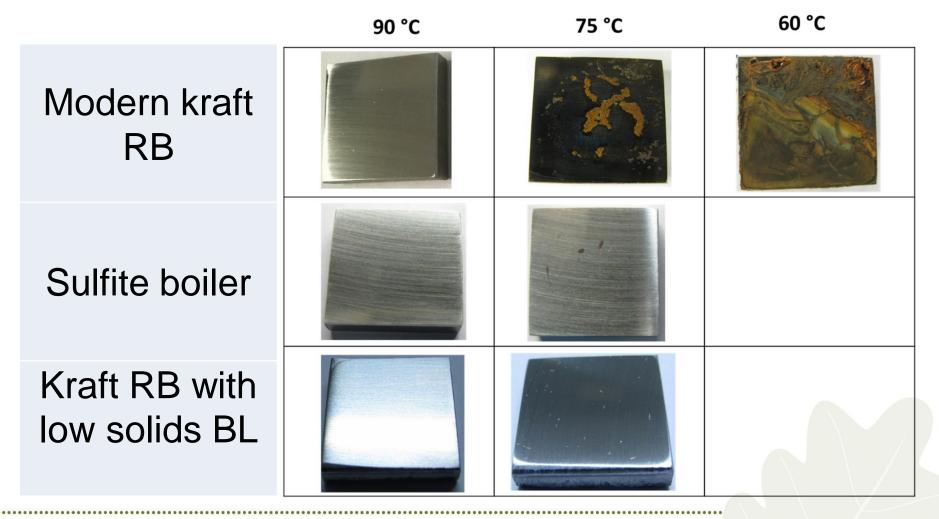
No corrosion seen at 90 °C
