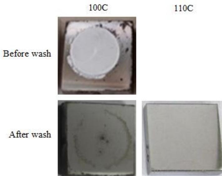
Figure 6. Na<sub>2</sub>SO<sub>4</sub> on carbon steel after 24h exposure with 60 vol% H<sub>2</sub>O.
