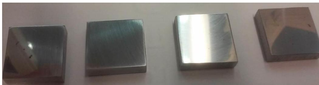
Figure 11. Precipitator ash 1 on carbon steel coupons after 24h exposure at 110 °C with 80 vol-% H<sub>2</sub>O.
