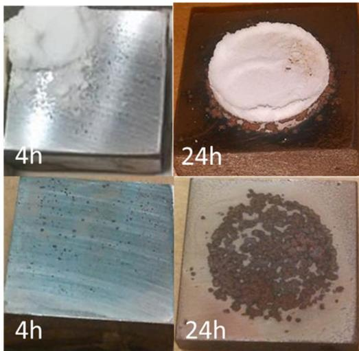
Figure 3. Samples under  $\text{Na}_2\text{SO}_4$  at 60%  $\text{H}_2\text{O}$  and  $100\text{ }^\circ\text{C}$  for 4h or 24h.
