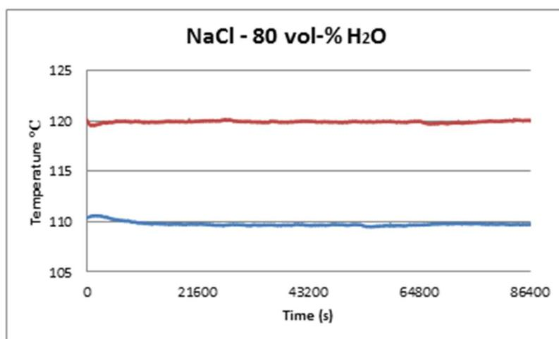
Figure 2. Temperature profiles for the experiments with NaCl at 110°C and 120°C, 24h run with 80 vol%  $\text{H}_2\text{O}$ .
