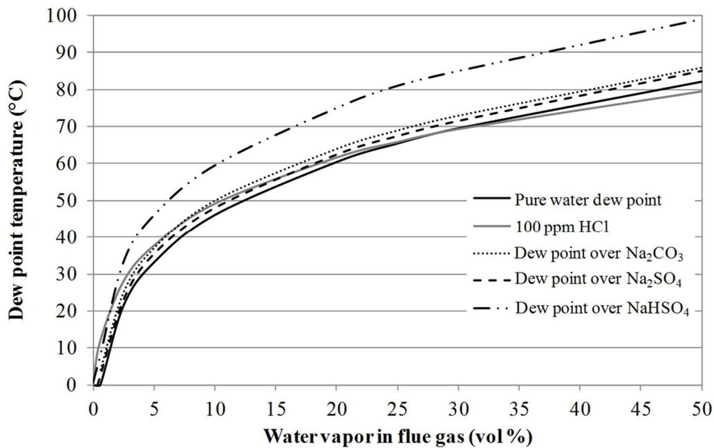
Figure 1. Pure water dew point, and humidity of deliquescence for the hygroscopic salts ( $\text{Na}_2\text{CO}_3$ ,  $\text{Na}_2\text{SO}_4$  and  $\text{NaHSO}_4$ ) as a function of water vapor concentration. Adapted from [2].
