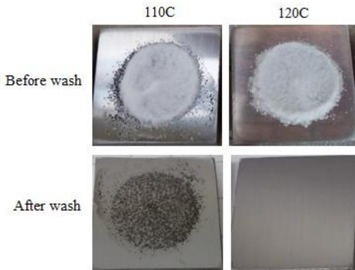
Figure 8. NaCl on carbon steel after 24h exposure with 80 vol%  $\text{H}_2\text{O}$ .
