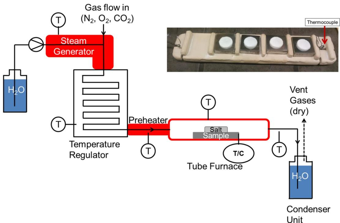
Figure 4. Experimental set-up used in this work.
