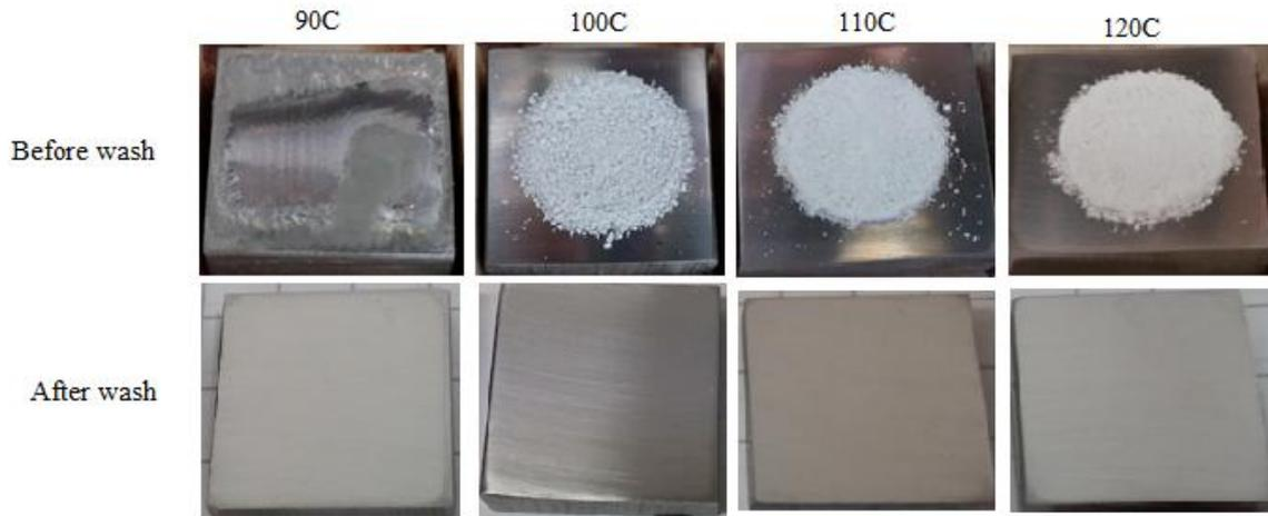
Figure 7.  $\text{Na}_2\text{CO}_3$  on carbon steel coupons after 4h (90°C and 100°C) and 24h (110°C and 120°C) exposure with 80 vol%  $\text{H}_2\text{O}$ . Sodium carbonate dissolved in absorbed water after 4h exposure at 90°C with 80 vol%  $\text{H}_2\text{O}$ .
