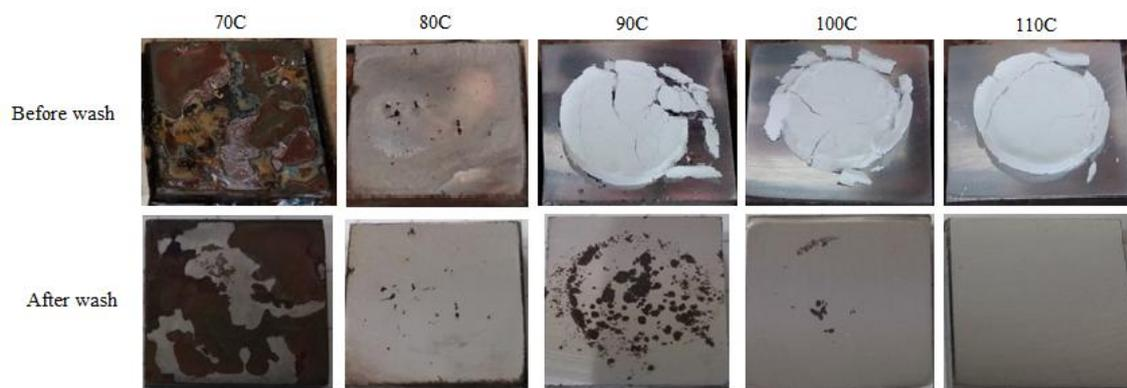
Figure 9. Precipitator ash 1, on carbon steel coupons after 24h exposure at 70°C to 110°C with 27 vol% H<sub>2</sub>O. The ash is dissolved in absorbed water at 70°C and 80°C.
