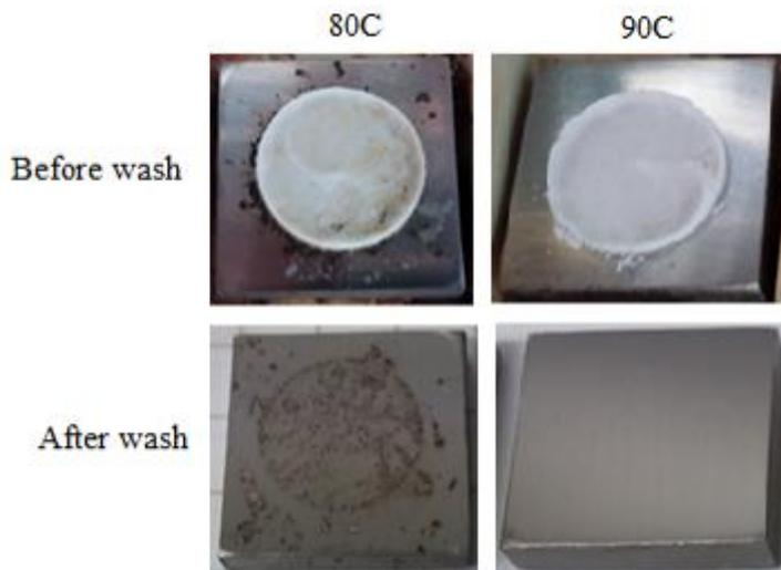
Figure 5. Na<sub>2</sub>SO<sub>4</sub> on carbon steel after 4h exposure with 27 vol% H<sub>2</sub>O.
