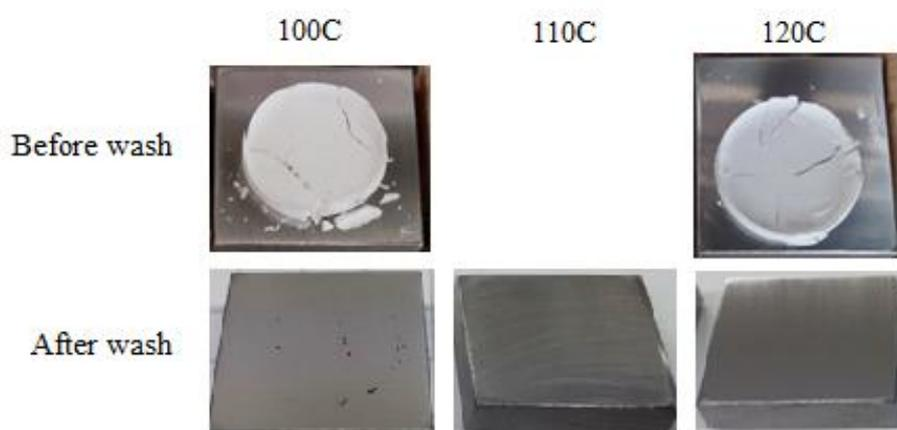
Figure 10. Precipitator ash 1 on carbon steel coupons after 4h exposure at 100°C to 120°C with 60 vol% H<sub>2</sub>O.
