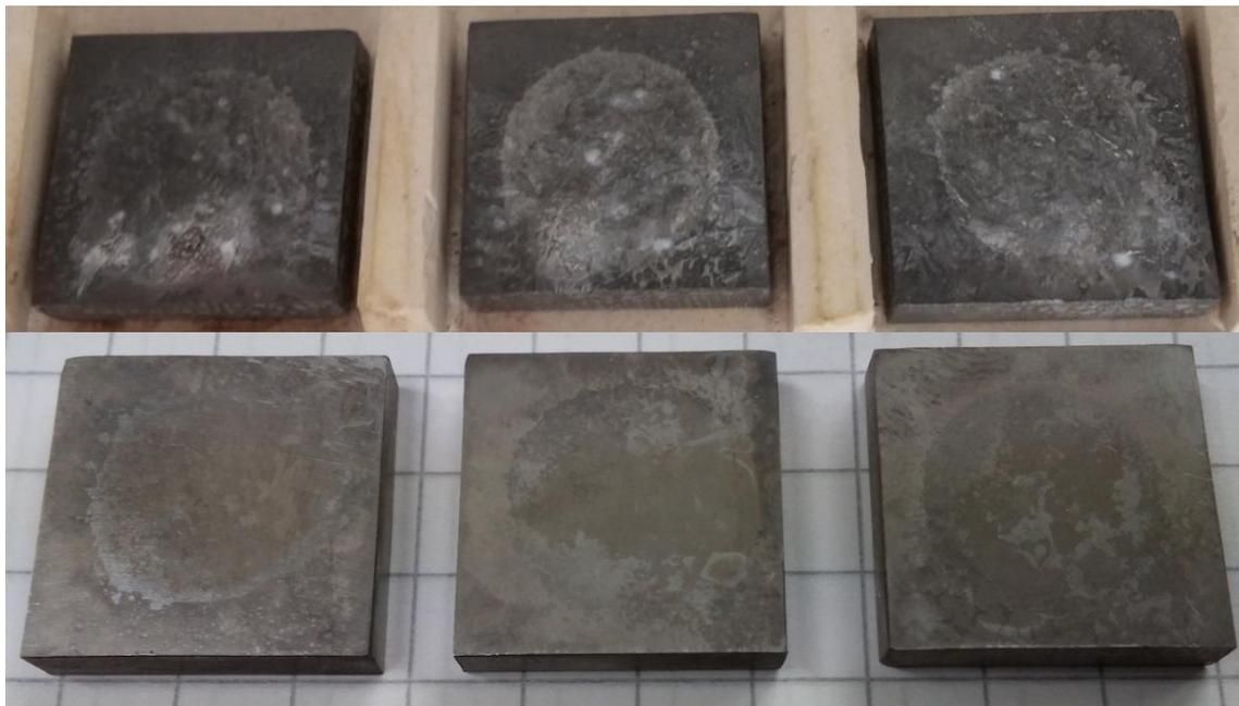
Figure 12. Unwashed coupons above and washed coupons below after 4h exposure to NaHSO<sub>4</sub> at 150°C and 60 vol%-H<sub>2</sub>O.
