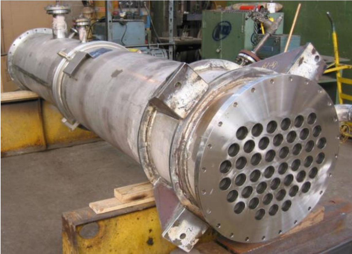
Figure 2.5. Evaporator tube bundle and tubesheet. Tube diameter is 5 cm (2 in.).
