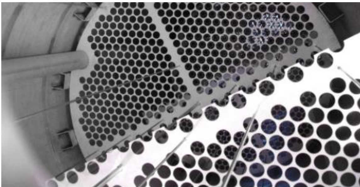
Figure 8. A distributor plate for tube type falling film evaporators for black liquor and other liquids [12].
