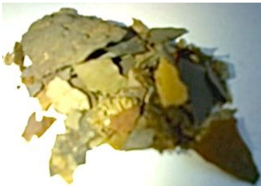
Figure 1. Flakes of aluminosilicate scale from a black liquor evaporator.
