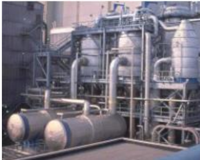
Figure 2.13. Photo of a forced circulation concentrator with two heat exchange loops [5].
