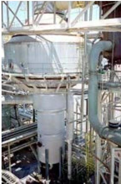
Figure 4. Photo of one body of a rising film evaporator.
