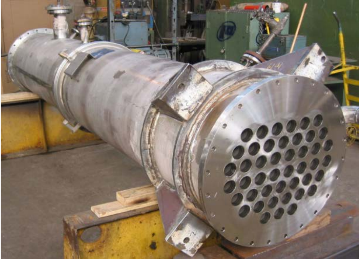
Figure 6. Evaporator tube bundle and tubesheet. Tube diameter is 5 cm.
