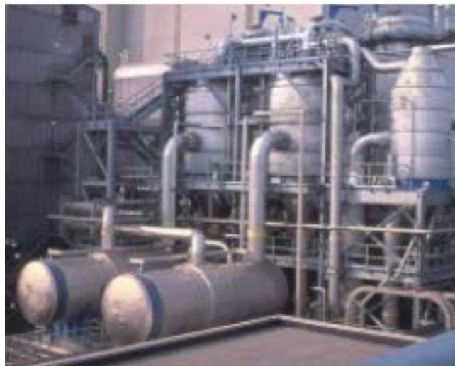
Figure 1-14. Photo of a forced circulation concentrator with two heat exchange loops. vii
