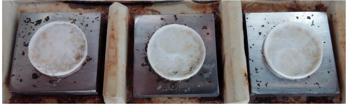
Unwashed coupons after 4h run at 80°C and 27 vol. % \text{H}_2\text{O} .
