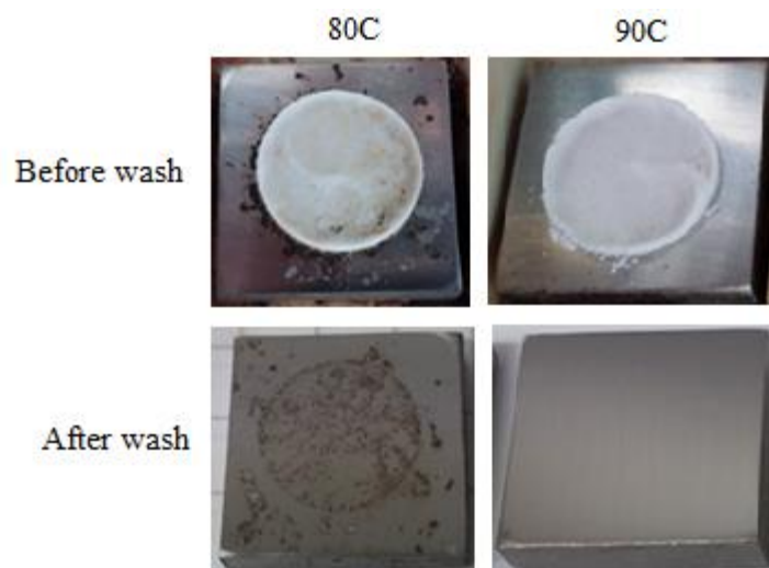
Figure 6.14. \text{Na}_2\text{SO}_4 on carbon steel after 4h exposure with 27 vol% \text{H}_2\text{O} .
