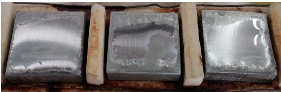
Figure 6.1. Sodium carbonate dissolved in absorbed water on carbon steel coupons after 4h exposure at 90°C with 80 vol% H 2 O. No corrosion could be detected.
