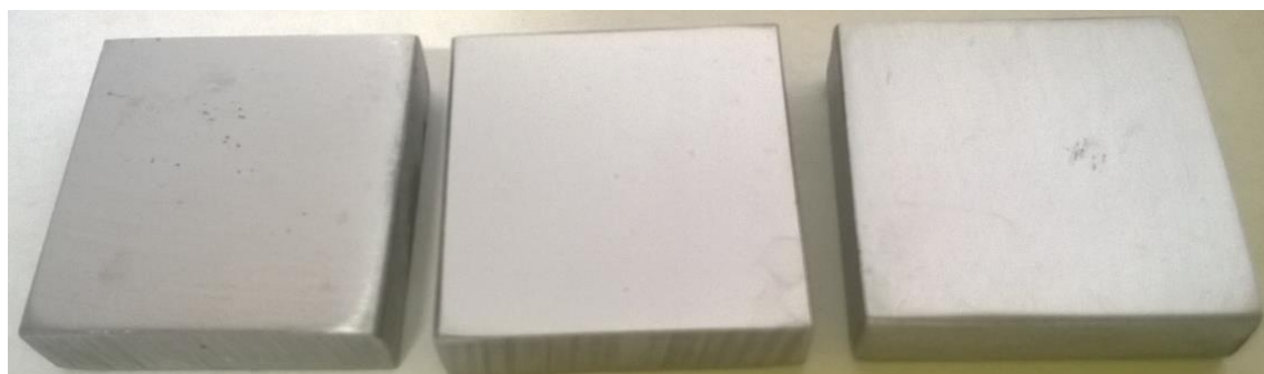
Washed coupons after 4h run at 100°C. Extremely weak corrosion in just a few sporadic spots. One coupon was taken to SEM/EDX analysis.
