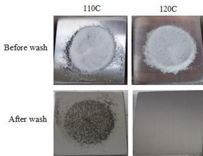
Figure 6.10. NaCl on carbon steel after 24h exposure with 80 vol% H 2 O.
