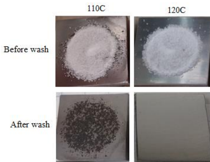
Figure 6.12. KCl on carbon steel after 24h exposure with 80 vol% H 2 O.
