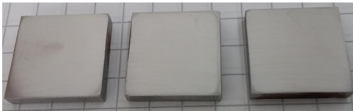
Washed coupons after 4h run at 120°C. No corrosion.
