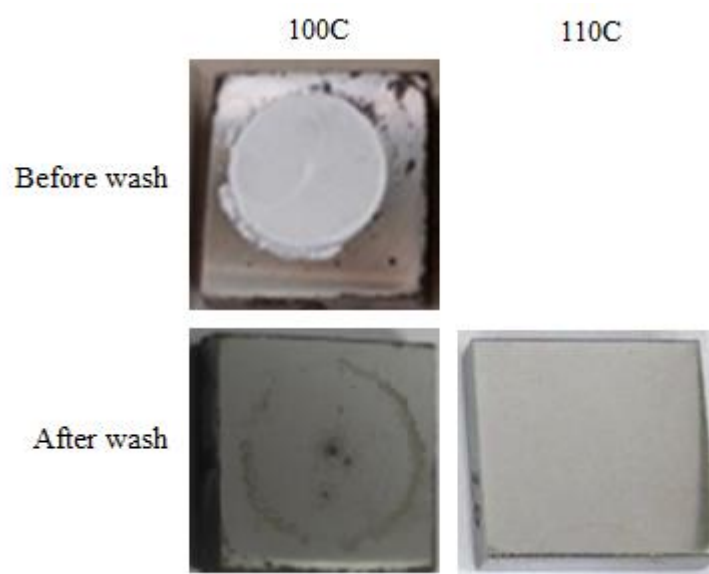
Figure 6.15. \text{Na}_2\text{SO}_4 on carbon steel after 24h exposure with 60 vol% \text{H}_2\text{O} .
