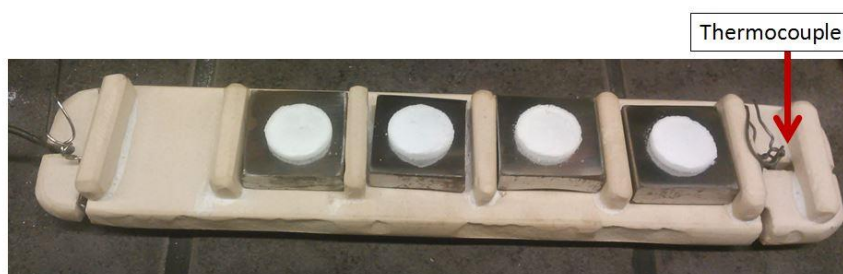
Figure 5.4. Carbon steel coupons with salt placed on the sample tray. The thermocouple was at the end of the sample holder.
