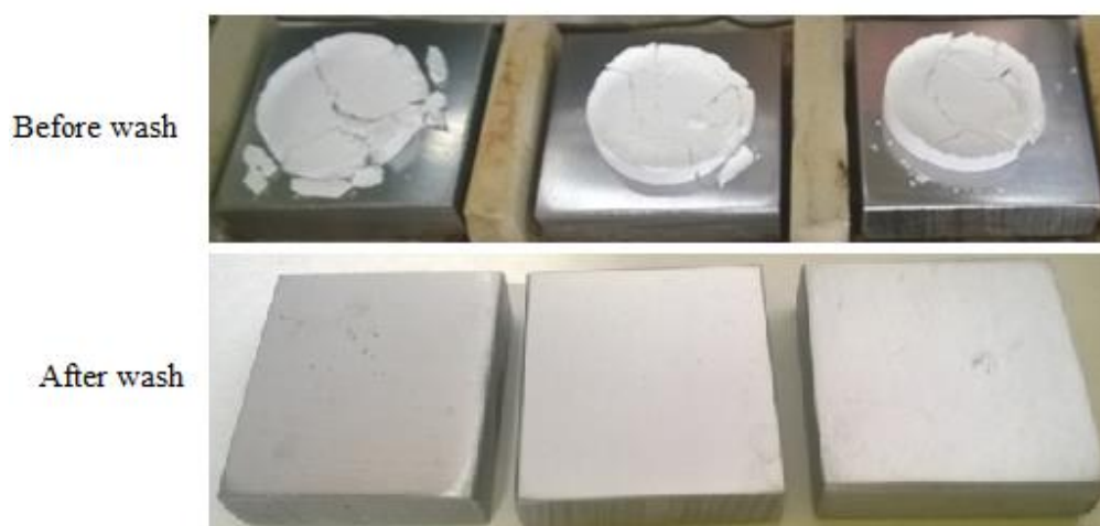
Figure 6.22. Precipitator ash 2 (PA2) on carbon steel after 4h exposure at 100°C with 27 vol% H 2 O. Possibly extremely weak corrosion categorized as insignificant and thus “no corrosion” at 100°C and 27 vol% H 2 O.
