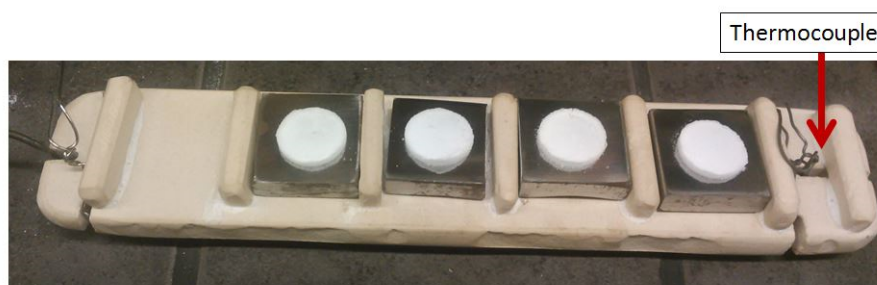
Figure 2. Carbon steel coupons with salt in top placed on the sample tray.
