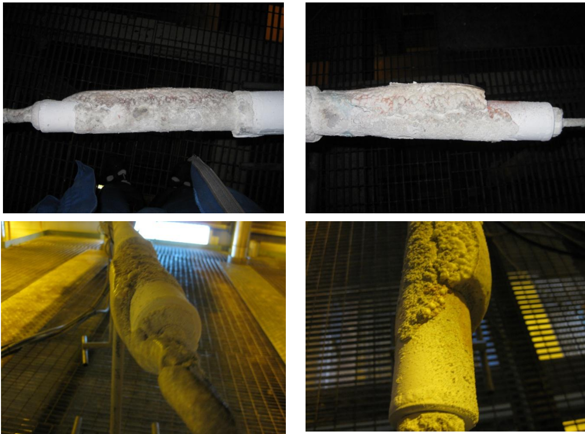
Figure 4. Post-exposure appearance of Probe 1 and Probe 2 shown in pictures in the left and right column, respectively.
