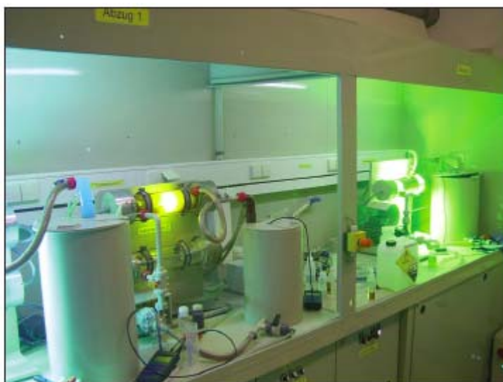
Photo 1: Laboratory scaled Enviolet® UV-plants (UV-reactors with different types of light sources)
