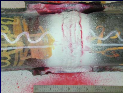
Butt Weld Cracking
