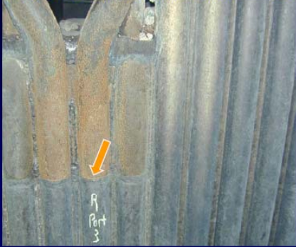
Finger Nail Corrosion – C.S.
