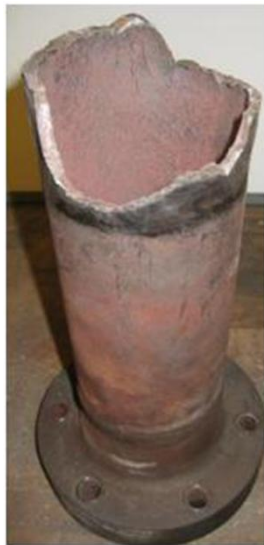
Broken lance 4 dm in from the rear flange
