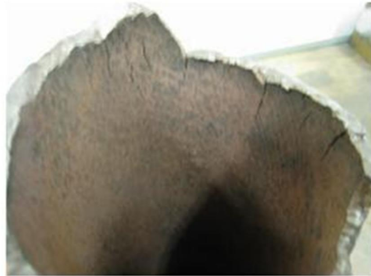
All cracks started from the inner side of the lances
