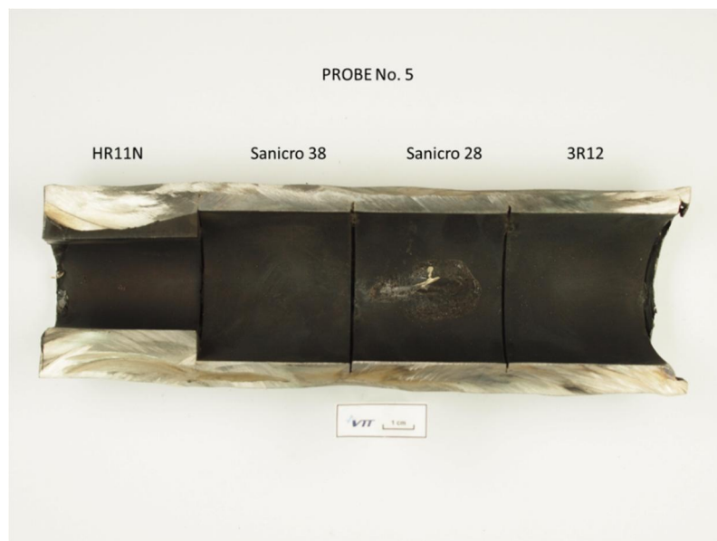
Figure 51. Macrographs taken from the probe No. 5 head after exposure: a) outer surface exposed to the furnace side and b) inner surface exposed to the cooling liquid. A thermocouple soldered on the middle of Sanicro28 specimen, that hindered WT measurements after exposure, is clearly visible on inner surface.
