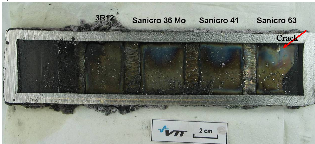
Figure 1. Separated probe samples a) after Test 3 cast in epoxy, and b) after Test 4.
