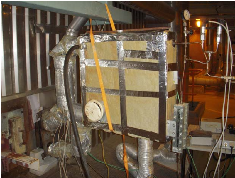
Figure 2. Experimental setup before installation into liquor gun opening.
