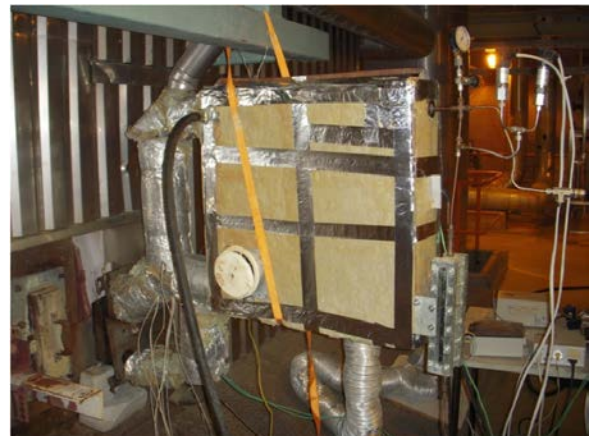
Probe before installation into liquor gun opening (MB Joutseno)
