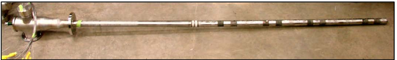
Probe for Crofton biomass boiler
