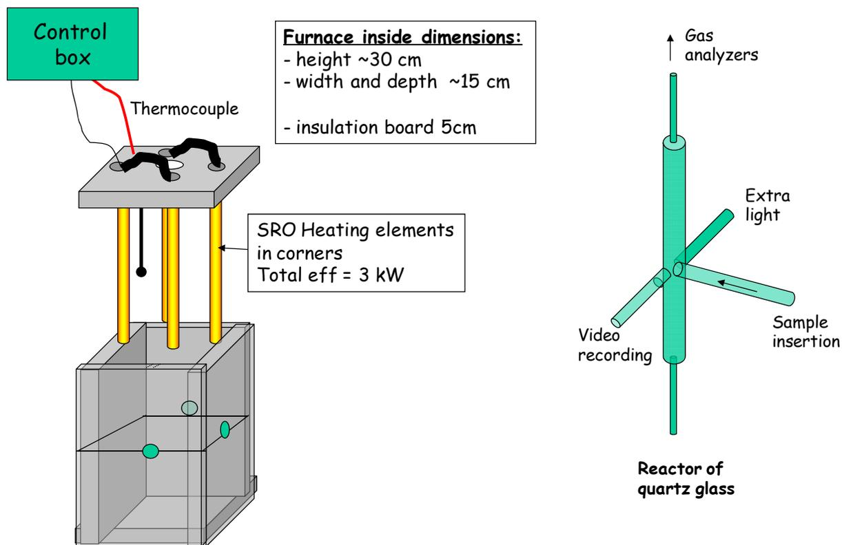
Figure 2. Reactor used for single droplet combustion tests.
