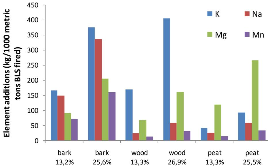
Figure 9. Rate of addition of elements per 1000 metric tons of black liquor dry solids fired.
