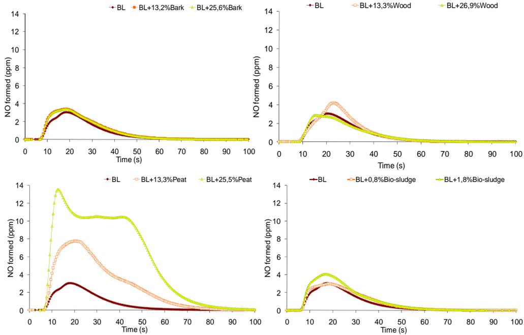
Figure 8. Average NO formation curves for the 6 droplets of the black liquor and mixtures.
