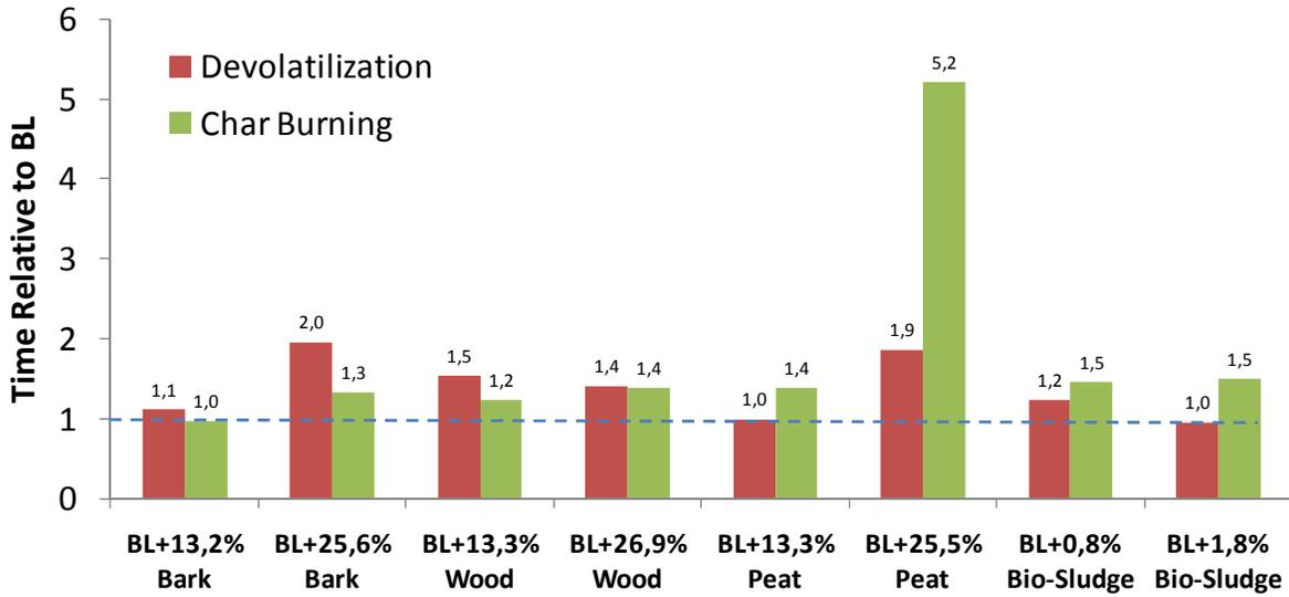
Figure 4. Relative devolatilization and char burning times for the black liquor and mixtures.
