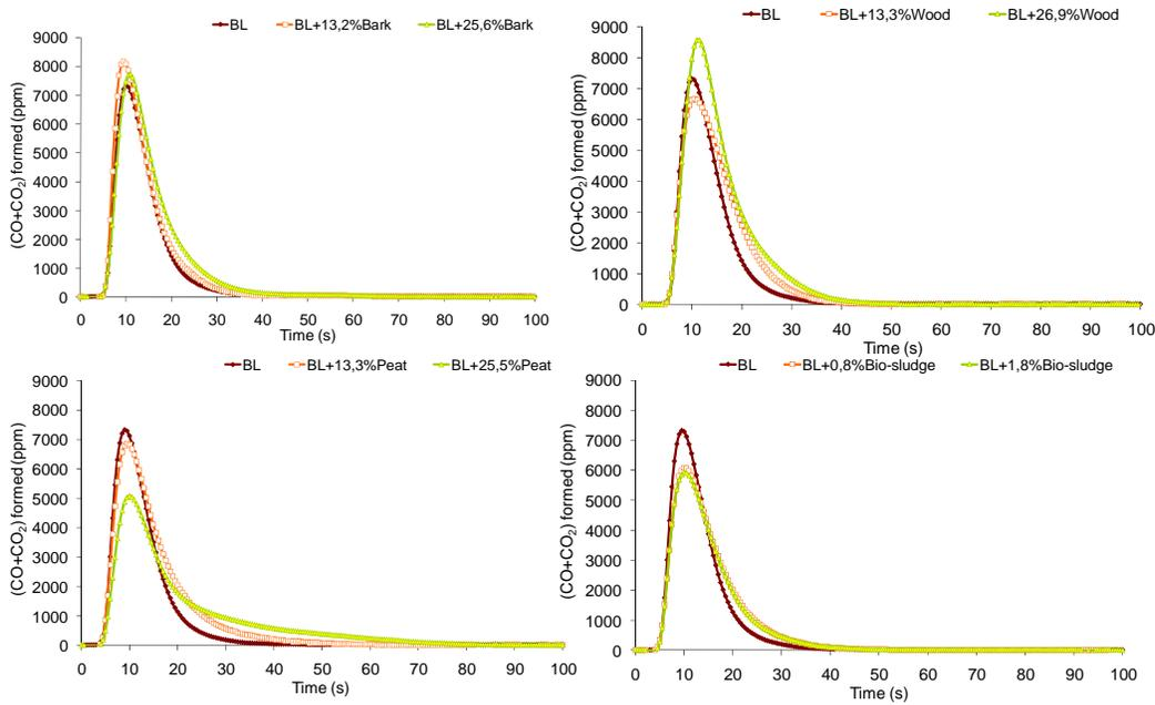
Figure 5. Carbon evolution as CO + CO<sub>2</sub> (avg. for 6 droplets) for the black liquor and the mixtures.
