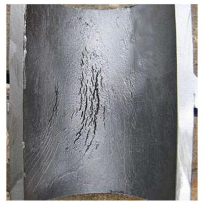
Fig. 1. Stress-assisted corrosion (SAC) damage in the internal surface of a 75 mm (3-in.) OD steel boiler tube with the scale removed to expose the crack-like damage.
