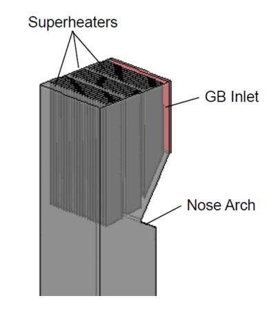
Superheater arrangement used for parametric evaluation
