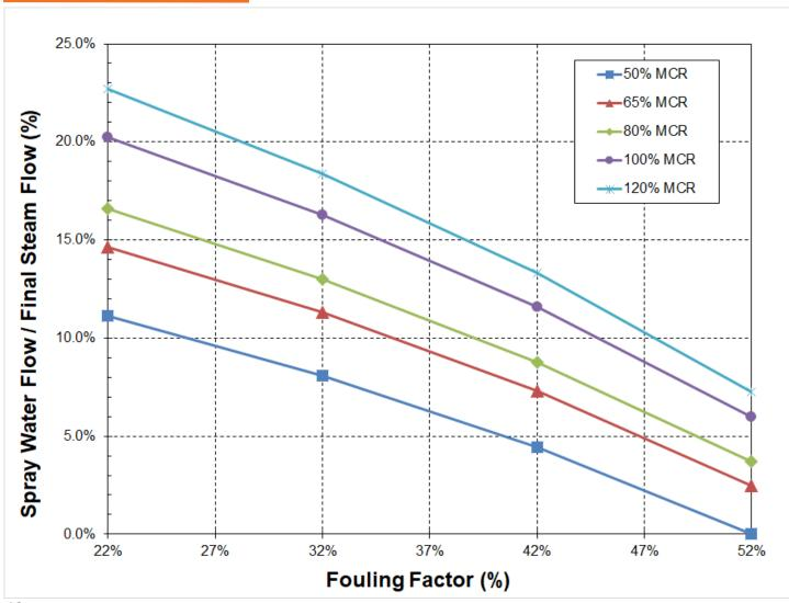
Higher PSH outlet steam temperatures lead to increased desuperheater spraywater demand
