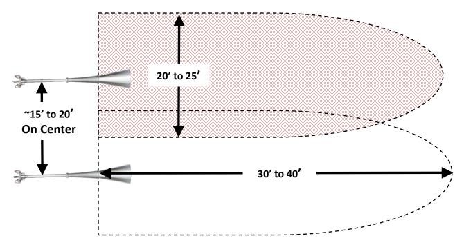
Note\* Cleaning patterns will vary based upon IMPULSE model used, as well as the temperature, boiler design, obstructions and internal components
