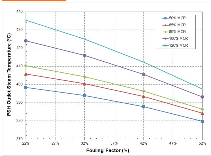
As fouling decreases below design level, heat transfer increases, leading to higher PSH outlet steam temperatures
