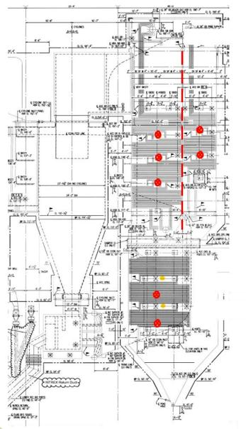
Two Identical 297.5 MW Foster Wheeler Circulating Fluidized Bed Combustors (CFBs) Burning a fuel-diverse mix of Petcoke, Coal, and Refuse.
