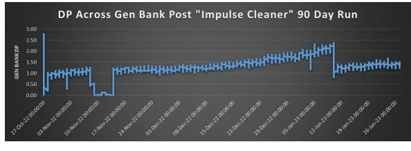
Following the installation of IMPULSE cleaners-Generating Bank after 90+ days of operation
