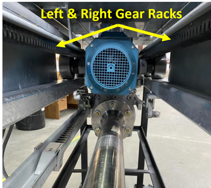
Both sides of the gear rack should wear at the same rate
