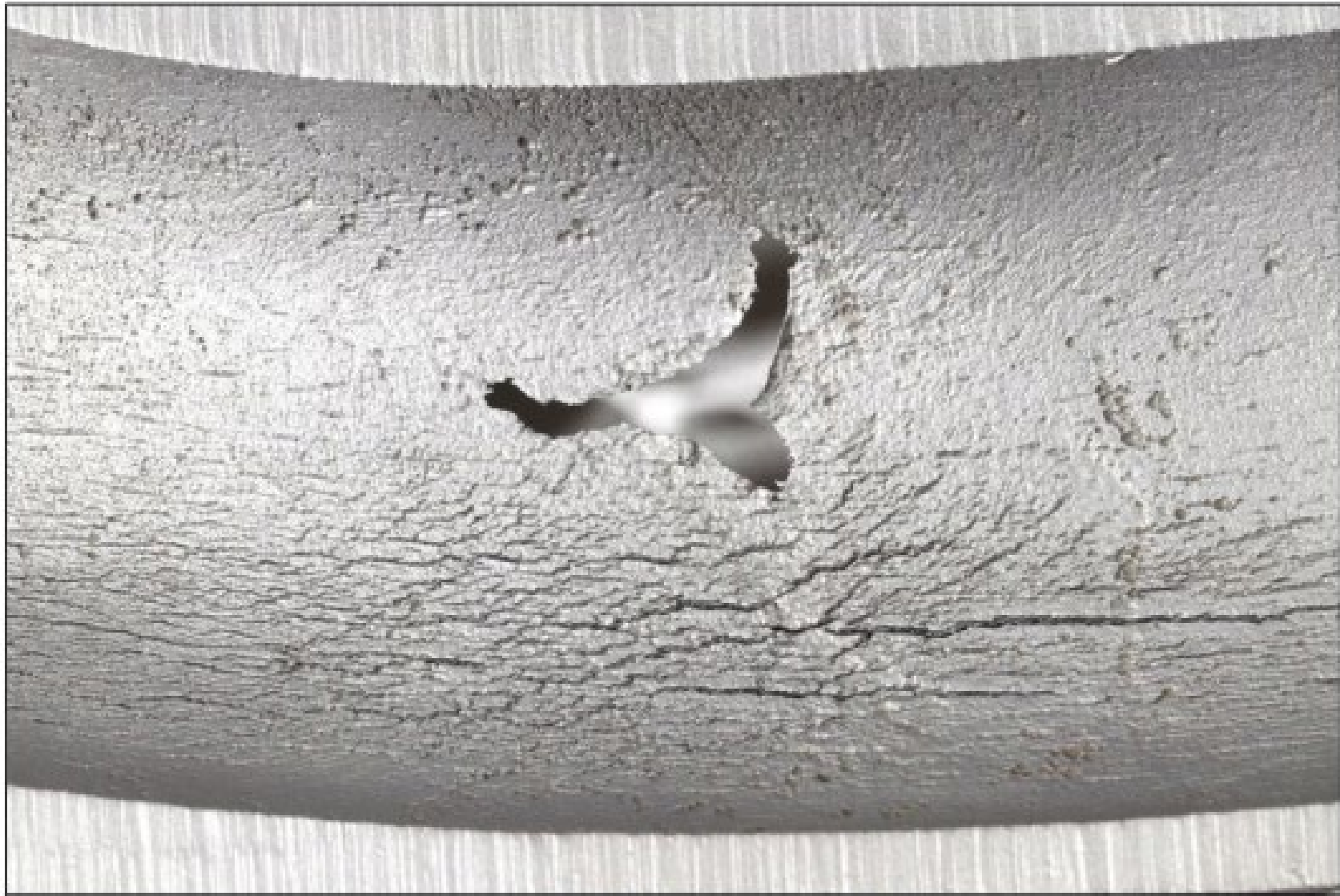
Figure 7 Failure location after cleaning. Significant SAC is present near failure location.
