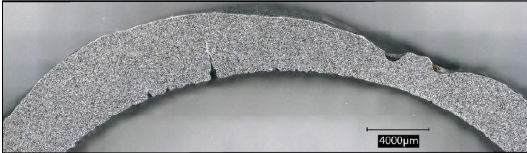
Figure 11 Cross section shows the SAC from the internal side adjacent to the external thinning.
