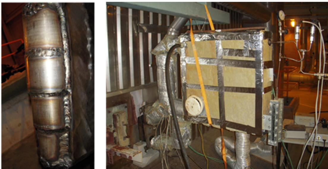
FIGURE 5-20. Steam generator front wall with tested materials and experimental setup before installation into liquor gun
