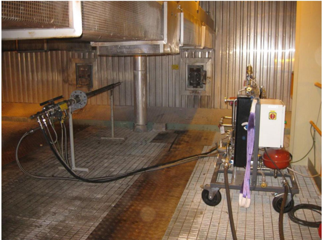
FIGURE 5-16. Probe ready for insertion through an inlet located about one meter below the sootblower at level 10½, between 2nd and 3rd superheater.
