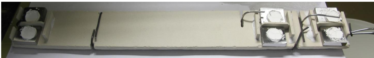
Figure 6. Sample holder used in the 1000h test. Note the thermocouples above the steel coupons. The samples at 120 °C are at the far left, the 100 °C samples are at the far right and the 105 °C samples are the samples in between.
