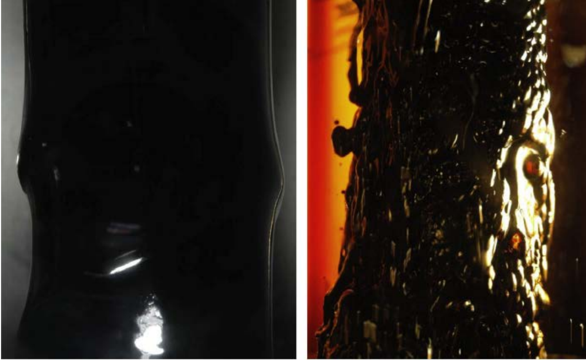
Figure 5. Hydrodynamic behavior of a black liquor falling film at q = 7700 , Re = 230 and Pr = 209 , (left) near the top of the evaporator tube, 0.3 m below the black liquor inlet, and (right) near the bottom of the tube, 4 m below the black liquor inlet. ix (From E. Karlsson et al., 2013.)
