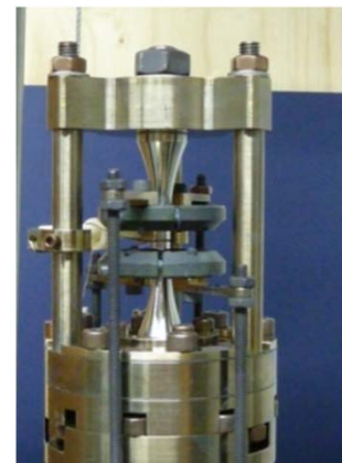
Pneumatic loading system (push / pull) based on bellows technology
