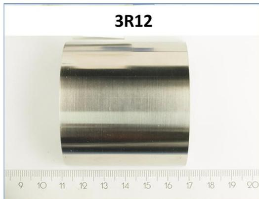
*Probe No. 4 - Surfaces machined and hand grinded/polished*
