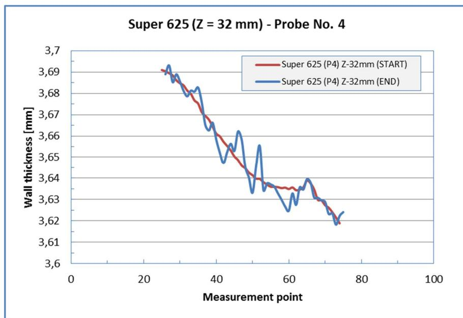
Figure 46. Circumferential wall thickness profiles from Super 625 specimen (Probe No. 4): a) axial location  $Z = 25$  mm and b) axial location  $Z = 32$  mm.
