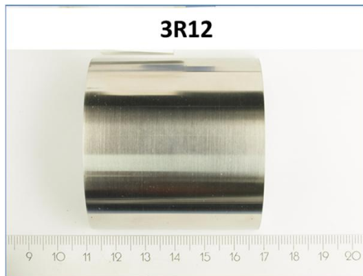
Probe No. 4 - Surfaces machined and hand grinded/polished
