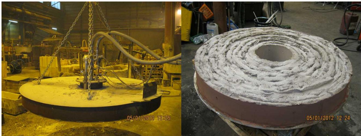
Figure 6. Old cover ready to use and new ladle heating cover just coated.
