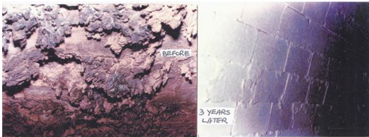
Figure 7. The effect of ITC coating on tunnel kiln buildup. (Courtesy of Feriz Delkic)
