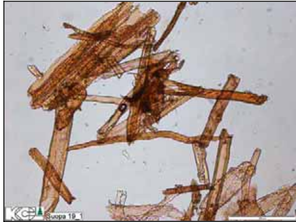
5.12. Kymi, acidulation feed soap (hydrochloric acid acidulation).
