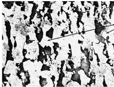
Superheater deposit (Straw)
