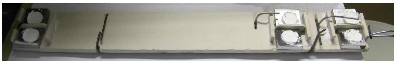
Figure 1. Sample holder used in the 1000h test. Note the thermocouples above the steel coupons. The samples at 120 °C are at the far left, the 100 °C samples are at the far right and the 105 °C samples are the samples in between.
