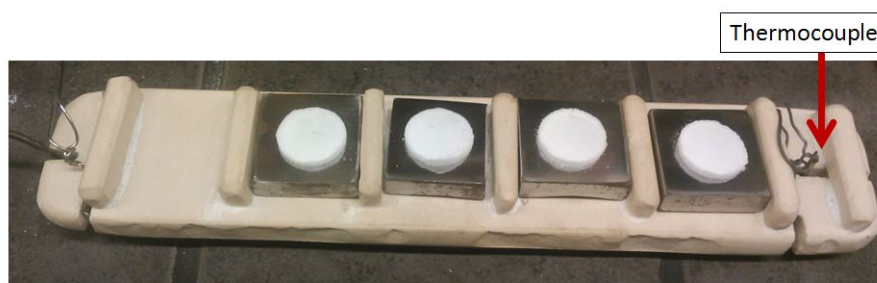
Figure 2. Carbon steel coupons with salt in top placed on the sample tray.
