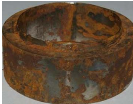
Figure 9. Ring after 1124h. Not that there are some areas without corrosion downwards on the bottom edge of the ring.
