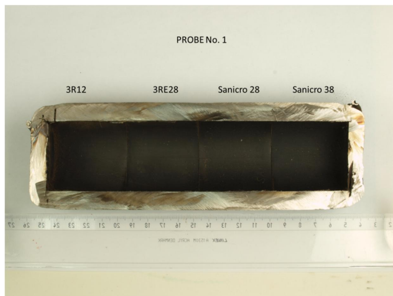
Figure 3. Macrographs taken from the probe No. 1 head after exposure: a) outer surface exposed to the furnace side and b) inner surface exposed to the cooling liquid.
