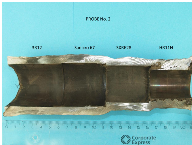
Figure 15. Macrographs taken from the probe No. 2 head after exposure: a) outer surface exposed to the furnace side and b) inner surface exposed to the cooling liquid.
