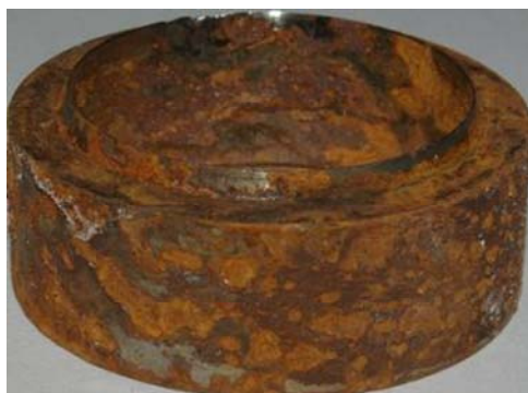
Figure 9. Ring after 1124h. Not that there are some areas without corrosion downwards on the bottom edge of the ring.
