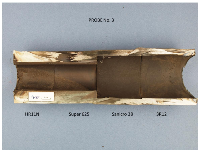
Figure 27. Macrographs taken from the probe No. 3 head after exposure: a) outer surface exposed to the furnace side and b) inner surface exposed to the cooling liquid.
