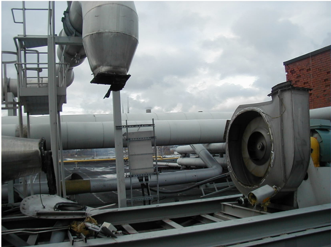
Figure 0-3. DNCG fan after the explosion.
