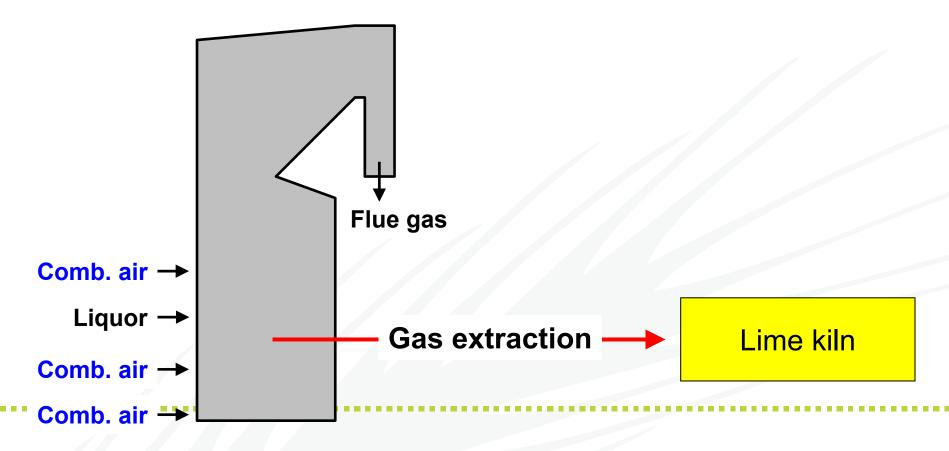
> Mass and energy balance calculations – cover needs of the lime kiln (30 MW) at a 500 000 ADt pulp mill
